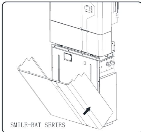
For Battery M4856-P, take out the front cover of M4856-P, and align the hole on the front cover with the power button on the battery body, then push it in place.
