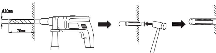
4. After cleaning the dust and other objects from the two holes, place 2 wall anchors into the holes, then attach the battery wall bracket to the wall by using the SW10 hexagon sleeve. Please use a level to ensure that the wall bracket is horizontal.
