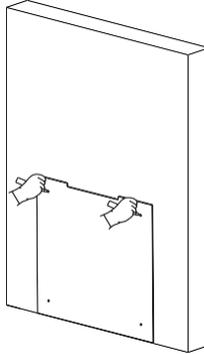
3. Drill 2 holes on the wall with a diameter of 10mm and a depth of about 70mm.
