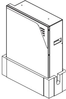
2. Place the battery positioning paper plate on the wall and stick the bottom to the floor, and mark the positions of the two drill holes.
