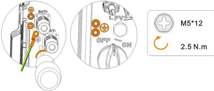
Connect the ground points between the battery and the inverter to ensure that the battery and the inverter have been grounded, as shown in the figure below.
