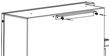
6. Place the battery against the wall, align the holes at the battery side to the screw holes of the wall bracket.
