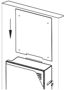
4) The bottom limit holes of the second battery will match the top screws of the first battery.
