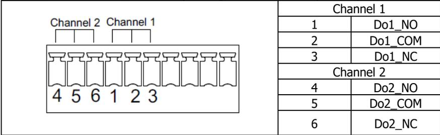
If using a generator unit with dry contact, the dry contact can be wired to 1 (Do1\_NO) and 2 (Do1\_COM) of Channel 1 as shown in the diagram below. If using a generator unit without dry contact, no wiring is required.
