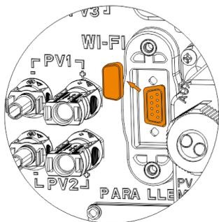
2. Tighten the Wi-Fi module onto the inverter with screw M4\*10 (X2)
