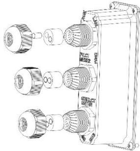
Unscrew the nut of cable gland and take out the rubber cylinders.
