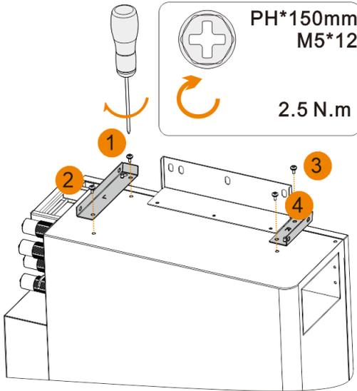
2. Attach the inverter to the mounting bracket. Mount the supporting bracket at the bottom of the inverter.
