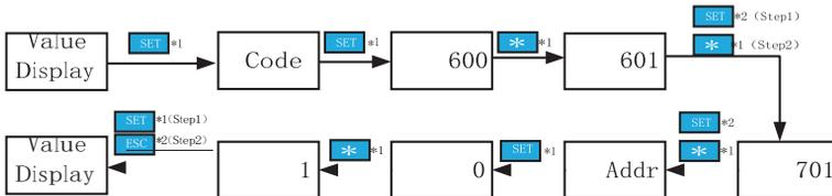
When the meter is used as PV meter, please follow the steps below to complete the address setting by pressing the corresponding button and the number of times.
